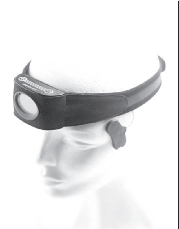
**Fig. 2.** Miniature self-contained EMG detector–analyser with biofeedback function (Grindcare<sup>®</sup>) (courtesy of Prof. Peter Svensson).
